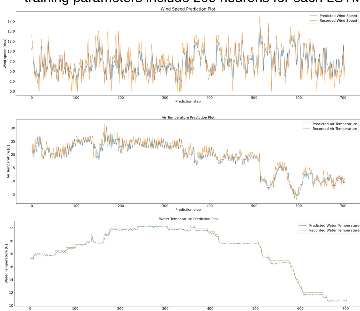
Fig. 3. Model estimation (red: recorded, blue: predicted) data for the testing dataset. The testing data is 10% from the actual data (Fig. 1).
