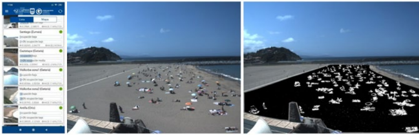
Fig. 6. A snapshot of the Nik Hondartzak app on the left. Centre, an image captured and on the right the result of the detection algorithm on Santiago-Zumaia beach, on 20 July 2020. The analysed region is in black.
