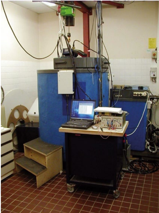
Fig. 2. Picture of the 800 l calibration bath.
