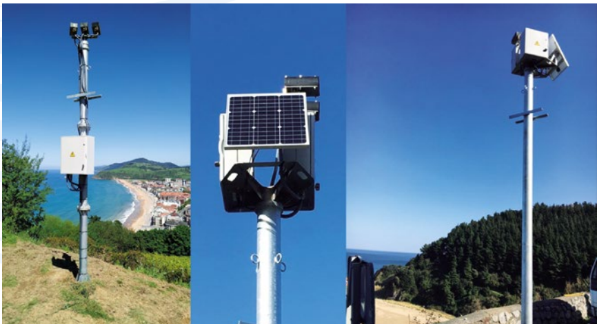
Fig. 1. KOSTASystem coastal videometry stations. From left to right, Zarautz station, and two views of a photovoltaic autonomous station in Saturrarán.
